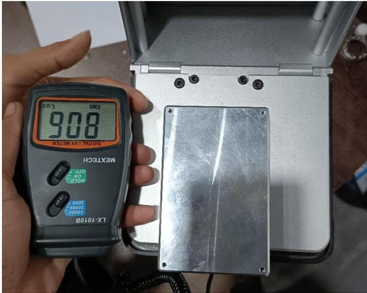
4. Measure the lux and adjust the value with calibration knob, which is given at the back side of the machine, with screw driver. (Rotate the knob clock wise to increase the lux value & anti clock wise to decrease the lux.)
